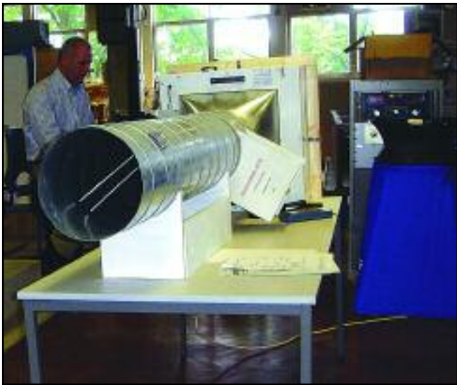
Air volume measuring rig with hood shown on the right
